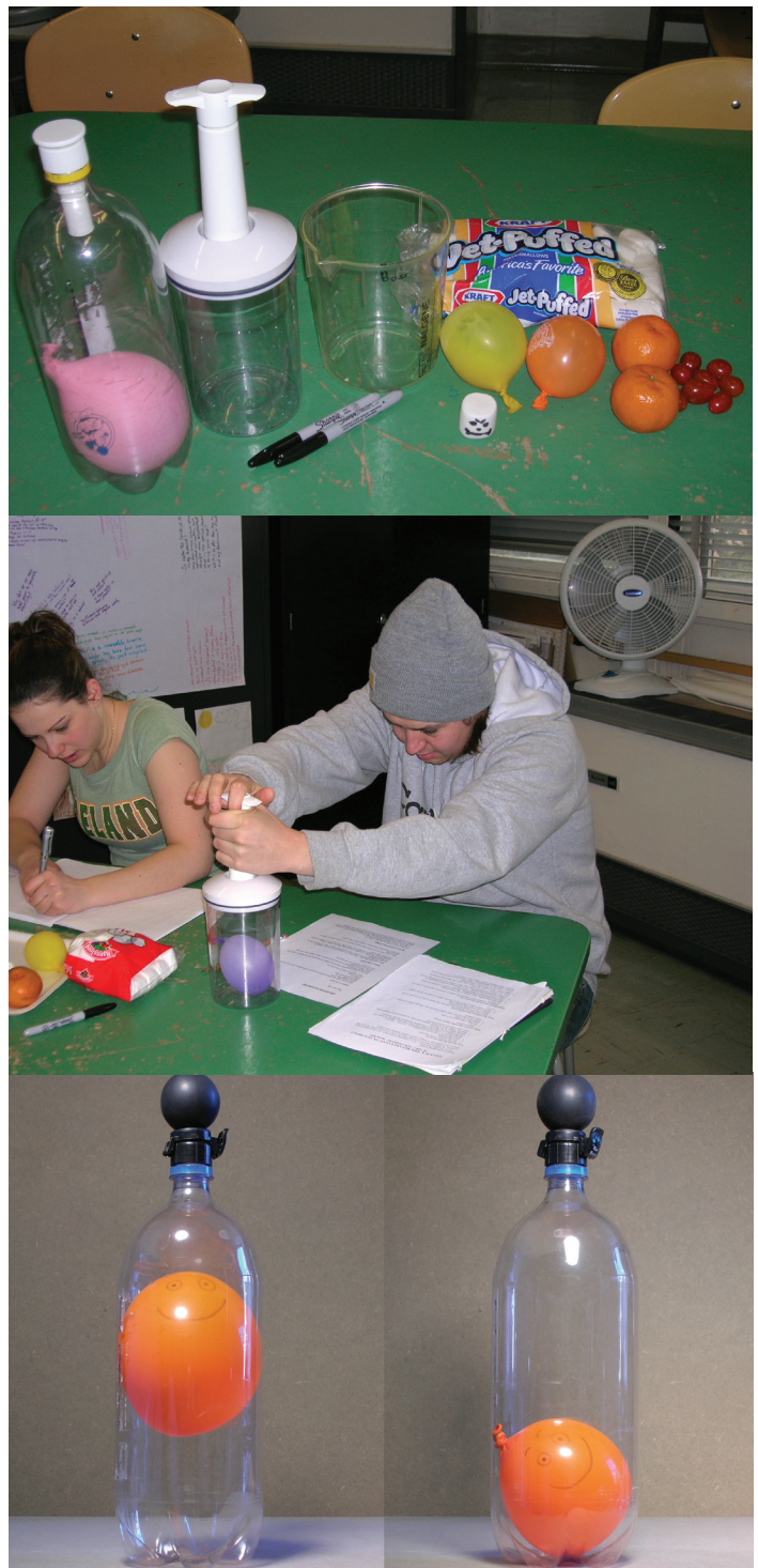
Figure 2.5. (top) Materials for Activity 2.5. (middle) Testing an air-filled vacuum container. (bottom) An air-filled balloon under atmospheric pressure (left) and after air was pumped into the bottle (pressure increased; right).
