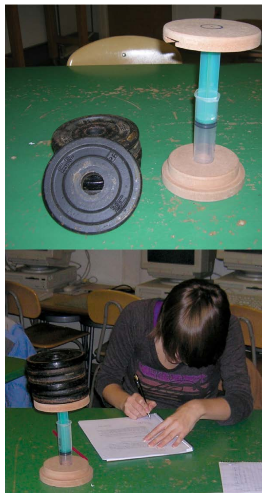
Figure 2.6. (top) Materials for Activity 2.6. (bottom) The apparatus once 15 lbs have been laid on its top.
