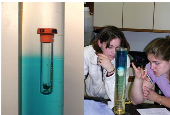
Figure 5.3. Buoyancy oscillations. An object of intermediate density rests between layers of dense bottom fluid and less-dense top fluid. If pushed down, the object will oscillate with a frequency dependent on the difference between fluid densities.
