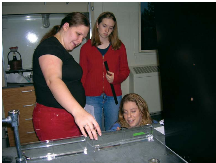
Figure 5.1. Wave speed and wave depth. Students measure the number of “sloshes” in a tank filled with water to a depth of 1.5 cm.
