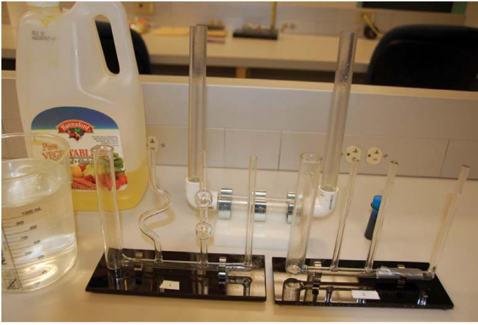
Figure 2.4. Materials used in Activity 2.4. The U-shaped manometer (Part A) is seen in the background. In the foreground is an equilibrium tube with different-shaped arms (left) and equilibrium tube with different arm diameters (right).
