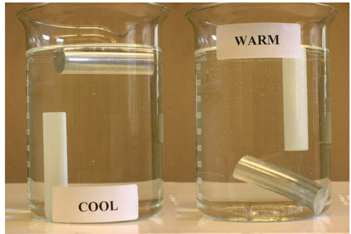
Figure 4.8. Aluminum and plastic rods immersed in cold and warm water.
