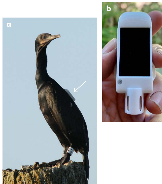
FIGURE 1. (a) A Brandt's cormorant ( Phalacrocorax penicillatus ) carrying a biologging device rests on a piling in the Columbia River Estuary, USA. Photo credit: A. Peck-Richardson (b) A biologging tag fitted with a fast-response temperature sensor and housing has proven useful. Photo credit: A. Peck-Richardson
