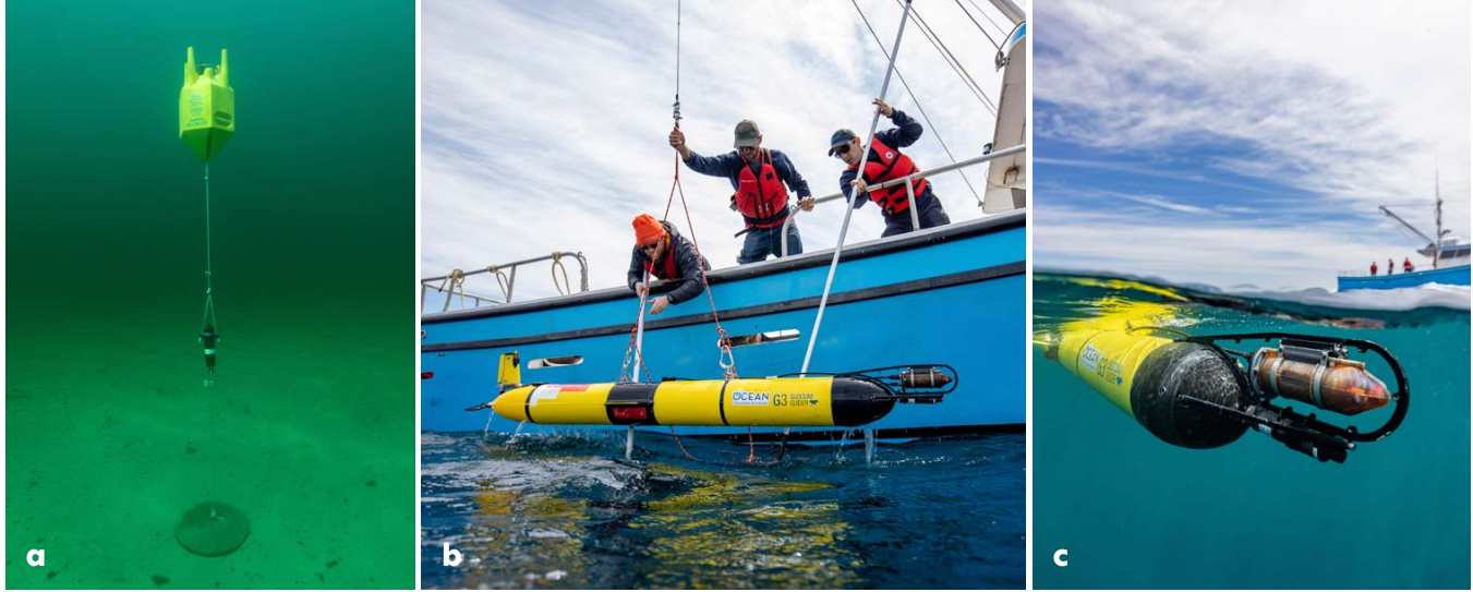
FIGURE 3. (a) Deployed acoustic receiver mooring (with sacrificial disc anchor, acoustic release, and yellow flotation collar housing the acoustic receiver) before deployment. (b) Recovery of a Slocum electric glider fitted at the bow with a Digital Acoustic Monitoring (DMON) external hydrophone to record whale calls. (c) Close up of DMON. Photo credits: Nicolas Winkler Photos courtesy of the Ocean Tracking Network
