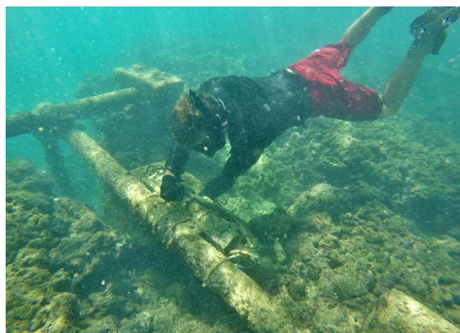
FIGURE 2. A diver maintains the water quality sensor at Kewalo Basin, O'ahu, which provided valuable data to the nonprofit organization Friends of Kewalos. Photo credit: PacIOOS
