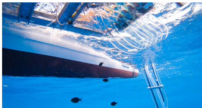
FIGURE 1. (above) The research catamaran floats peacefully in calm Fijian waters. This remotely piloted vehicle utilizes, among other things, a "skimmer" (right)—a rotating glass disk that skims the sea surface microlayer, sampling just the top 1 mm of the ocean. Photo credit: Alex Ingle/Schmidt Ocean Institute
