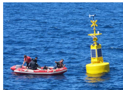
FIGURE 1. This moored buoy was installed on October 7, 2016, offshore Dakhla, southern Morocco to collect meteorological and oceanographic data. It has been out of commission since early March 2017 due to vandalism.
