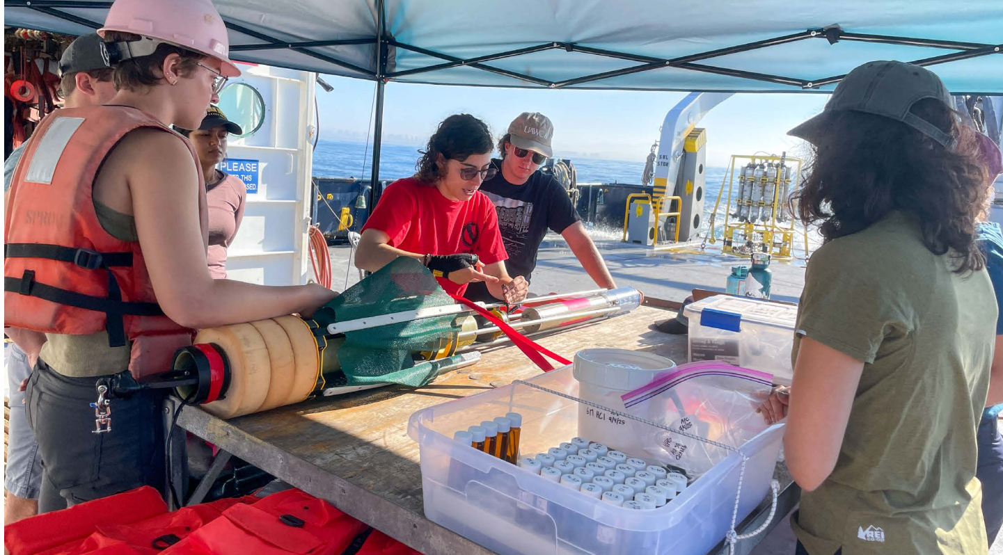
FIGURE 4. A graduate student instructor demonstrates epsilon meter setup for course participants while at sea.
