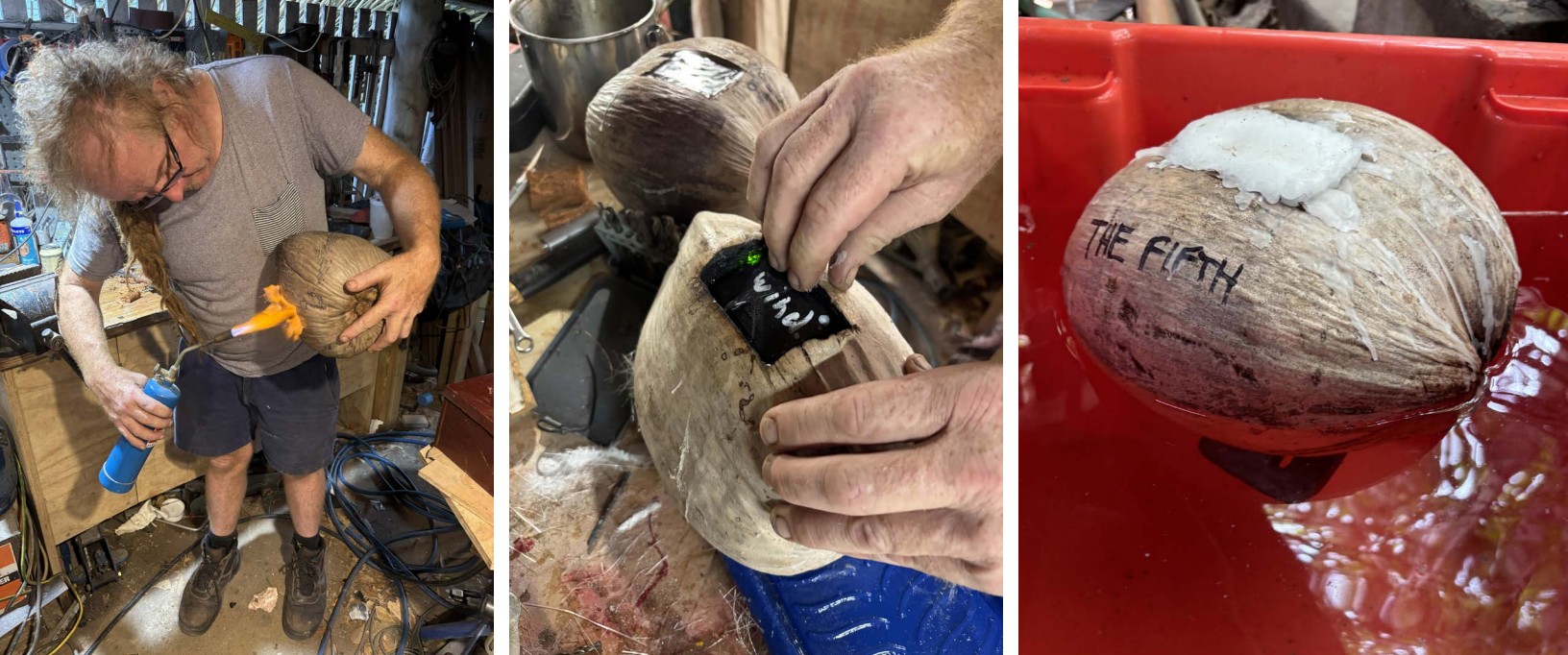
FIGURE 1. Coconut drifter fabrication. After the aperture was heat sealed (left), the tracker was inserted, with the signaling side facing up, into the paraffin wax-coated cavity (middle), and then ballasted using found, recycled, non-plastic materials (right). Image credits: Suzanne Long/RRRC
