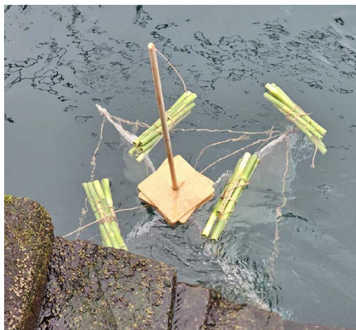
FIGURE 5. Before installing the GPS units, students tested the buoyancy and survivability of the drifter in ocean water along a loading dock. Students used the results of these tests to adjust buoyancy devices.
