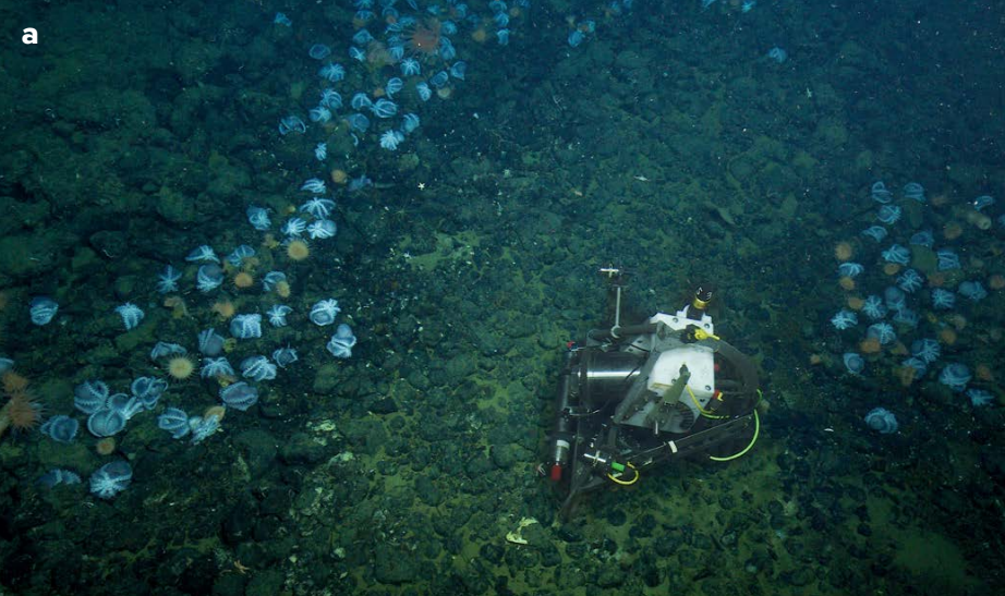
FIGURE 10. High-resolution mapping and imaging of the Octopus Garden (Figure 9) provided the basis for conducting targeted studies of the animals utilizing that habitat (Barry et al., 2023). In one instance, a time lapse camera was deployed from a ship on an ROV and then deposited precisely among benthic fauna where it operated autonomously (a). Still images from that vantage point were taken every 20 minutes from March 3, 2022, to August 29, 2022, revealing animals arriving, nesting, or dying post-breeding (b). The time lapse imagery provided a unique perspective on the dynamics of the community from scientific as well as educational and outreach purposes (Secrets of the Octopus Garden). Watch the video in the flipbook version of this article. Images © 2022 MBARI
