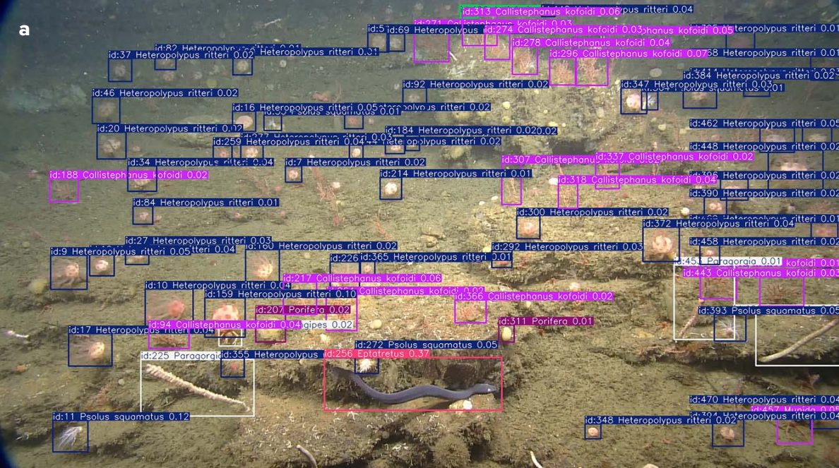
FIGURE 6. Videos are processed using an integration of MBARI's Video Annotation and Reference System (VARS) with advanced machine learning tools (VARS-ML) to identify and track animals (a) on the seafloor and (b) in the water column. The VARS-ML initiative combines the expertise of marine scientists, engineers, and data scientists. Watch the videos in the flipbook version of this article . Source: Lonny Lundsten and Nancy Jacobsen Stout. Images © 2025 MBARI
