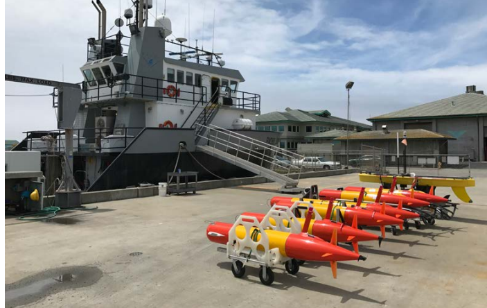
FIGURE 7. A fleet of long-range autonomous underwater vehicles (AUVs; Hobson et al., 2012) fitted with different imaging, water sampling, and eDNA collection payloads are lined up alongside a Liquid Robotics Wave Glider, all readied for deployment in Monterey Bay. The fleet of vehicles allows coordinated observations for extended periods to provide a multifaceted view of dynamic ecosystem processes. After Zhang et al. (2021a,b). Susan von Thun © 2017 MBARI
