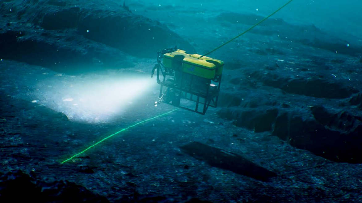
FIGURE 8. Animation demonstrates the combined use of ship, AUV, and ROV-based surveys to obtain high-resolution seafloor bathymetry and imagery at Sur Ridge within the Monterey Bay National Marine Sanctuary (Seeing Sur Ridge). Watch the animation in the flipbook version of this article. © 2023 MBARI
