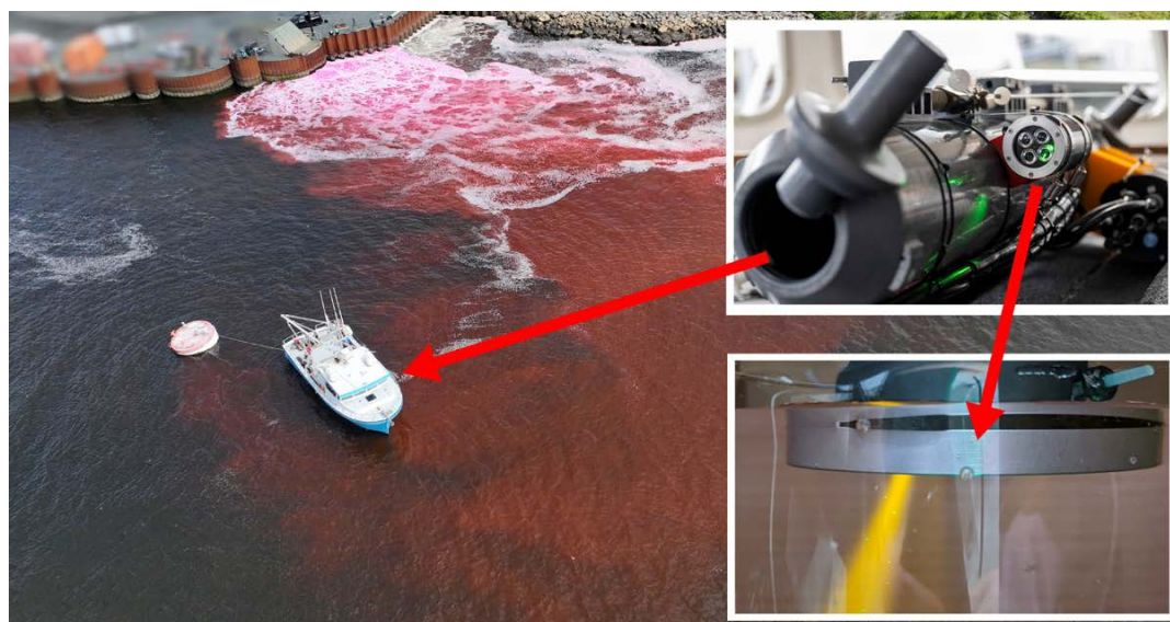
FIGURE 1. Drone photograph of the August 2023 Halifax Harbor tracer release experiment conducted from the diving vessel Eastcom. Insets: The PIXIE open-source fluorometer is shown mounted to the side of a Niskin bottle (top) and during rhodamine water tracer (RWT) calibration (bottom) in the lab.
