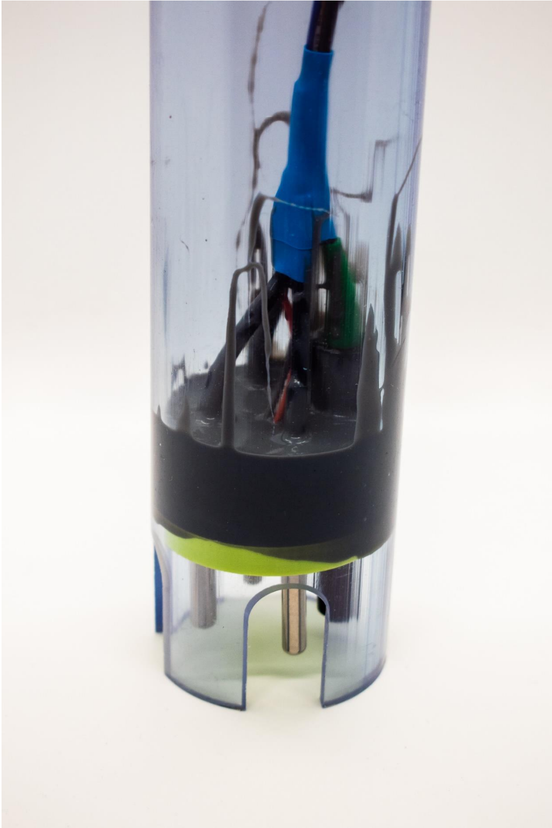
Figure 18. A clear OpenCTD showing the thick epoxy potting layer.
