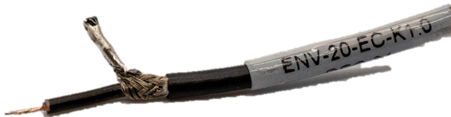
Figure 14. Conductivity probe leads with coaxial wires stripped and soldered.
