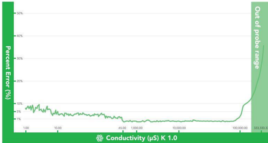
Figure 24. Accuracy of Atlas Scientific K 1.0 Conductivity Probe and EZO circuit. Data provided by Atlas Scientific.
