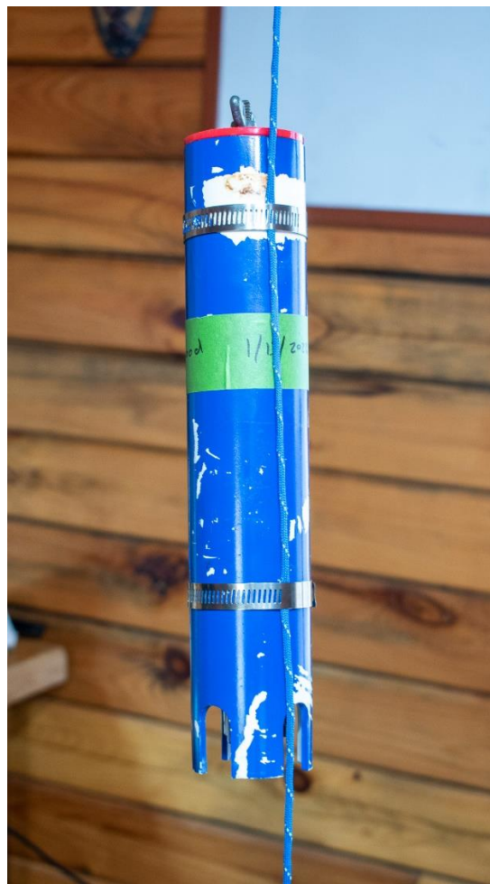
Figure 29. Example of OpenCTD attached to weighted anchor line using hose clamps.
