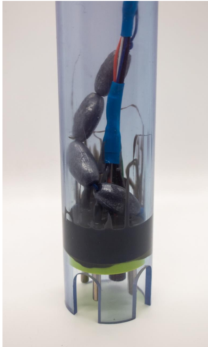
Figure 30. Clear OpenCTD with fishing weights inside.
