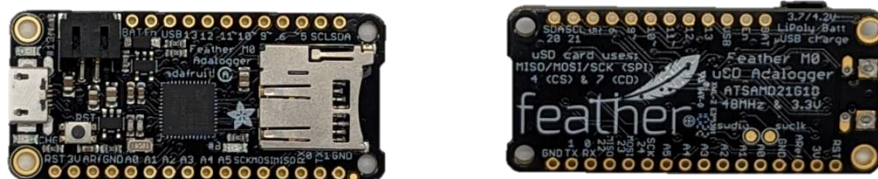
Figure 4. Adalogger M0 without headers. Left: topside of the board. Right: bottom of the board.
