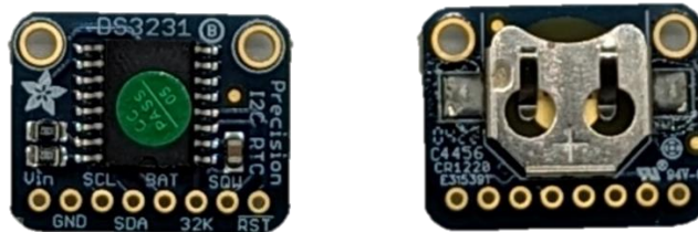
Figure 8: Real-Time Clock module without headers. Left: chip side of the board. Right: battery side of the board.
