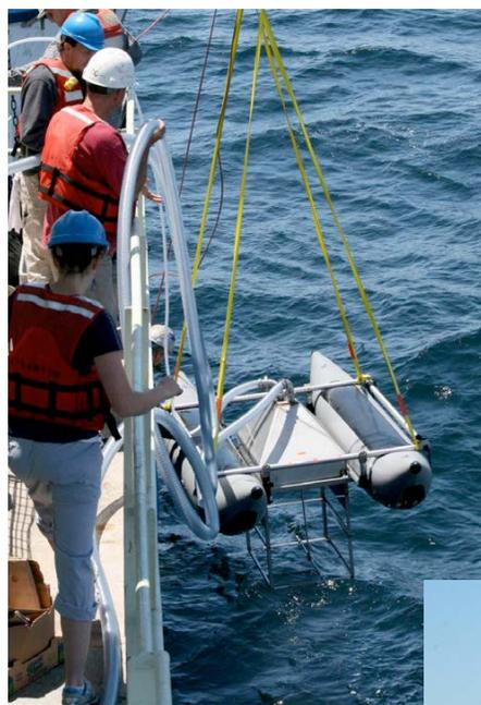
**FIGURE 4.** Deployment of Sea Sweep from Woods Hole Oceanographic Institution's R/V *Atlantis* off the coast of California.
