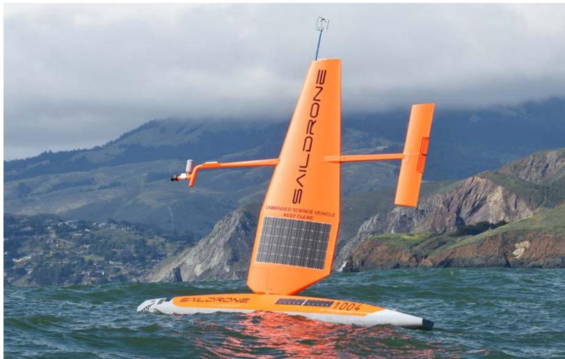
**FIGURE S1.** Example of an autonomous surface vehicle with a sail deployed off the coast of California, USA (Meinig et al., 2019). Saildrones and other autonomous ocean vehicles deployed in Earth's ocean typically carry payloads with a variety of environmental sensors. The example saildrone pictured here has in the past been equipped with a hull-mounted hydrophone, while other passive acoustic monitoring projects are planned that will deploy a hydrophone via a winch mechanism and soft tether.
