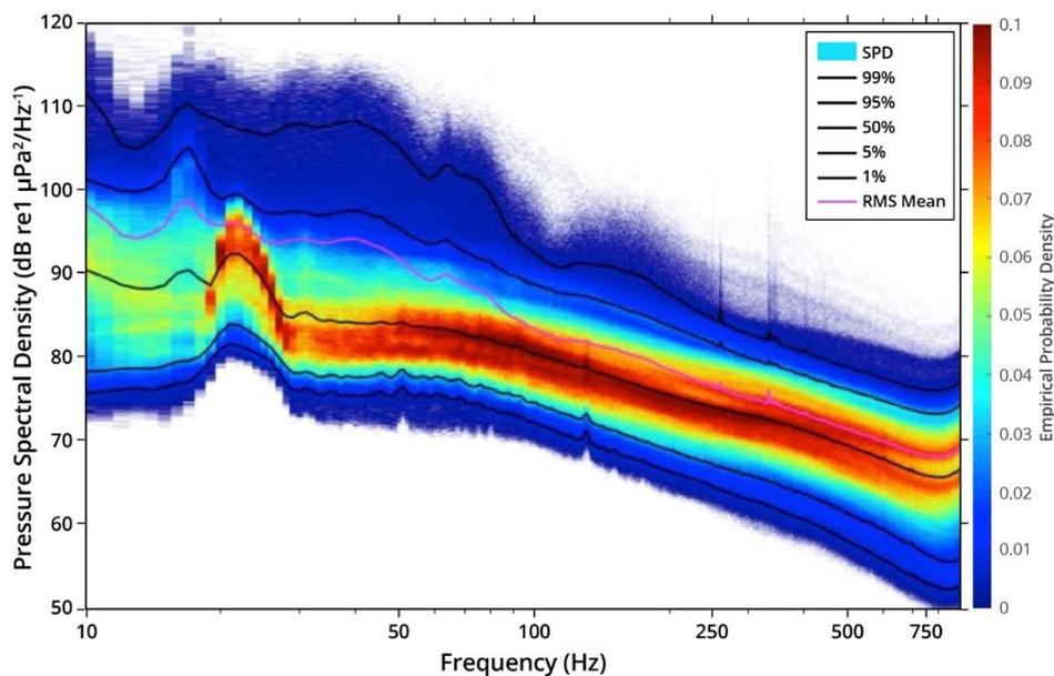
**FIGURE S3.** Spectral probability density (SPD) plot for one year of data collected in the European Arctic. The sound levels representing the 1<sup>st</sup>, 5<sup>th</sup>, 50<sup>th</sup>, 95<sup>th</sup>, and 99<sup>th</sup> percentiles of the soundscape are shown. The spectral peaks at 20–30 Hz (up to 50% of background sound levels) are the vocalizations of fin whales within the recording range of the hydrophone.
