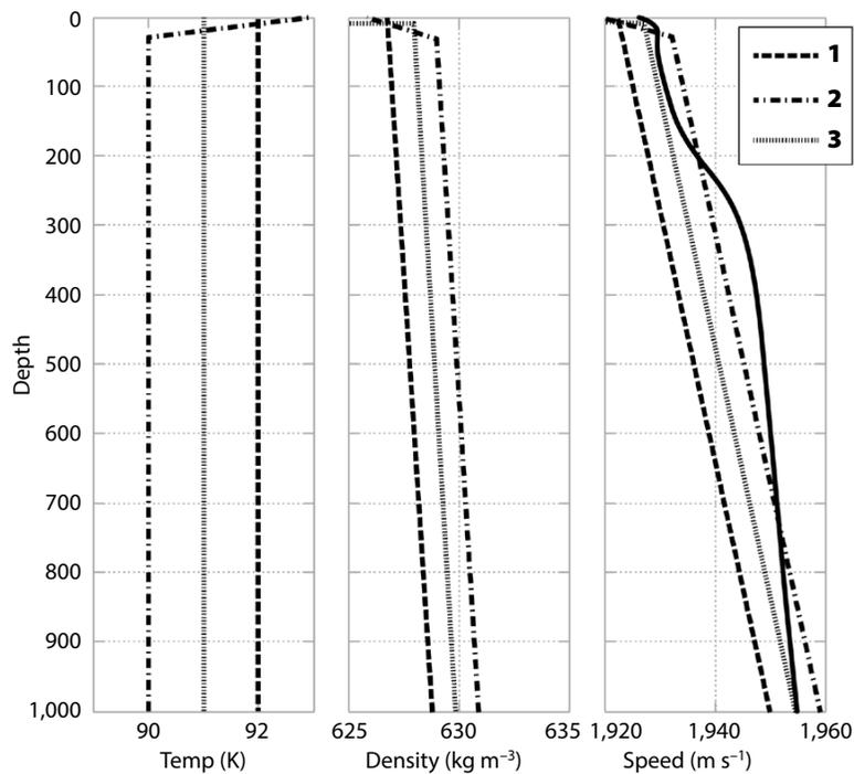
**FIGURE S2.** Depth profiles of temperature, density, and sound speed for the (1) isothermal, (2) thermally stratified, and (3) freshwater pool cases. A typical Arctic sea sound speed profile shifted by  $490 \text{ m s}^{-1}$  is included as the solid curve for comparison. After Arvelo and Lorenz (2013)
