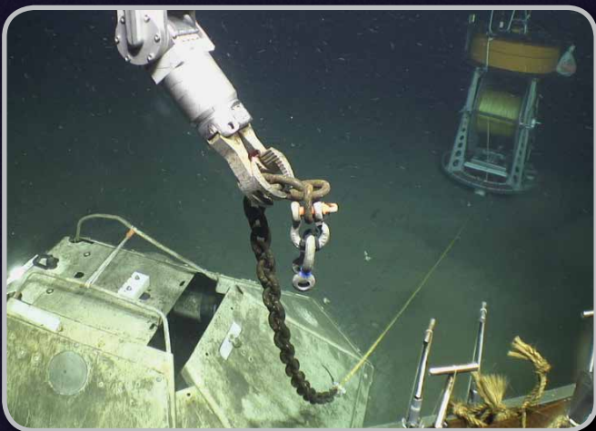
Figure 3. Underwater image of Jason attaching a chain and line from the “elevator” (upper right) to one of the ocean bottom seismometers (inside the trawl-resistant mount,) to facilitate the instrument’s recovery.
