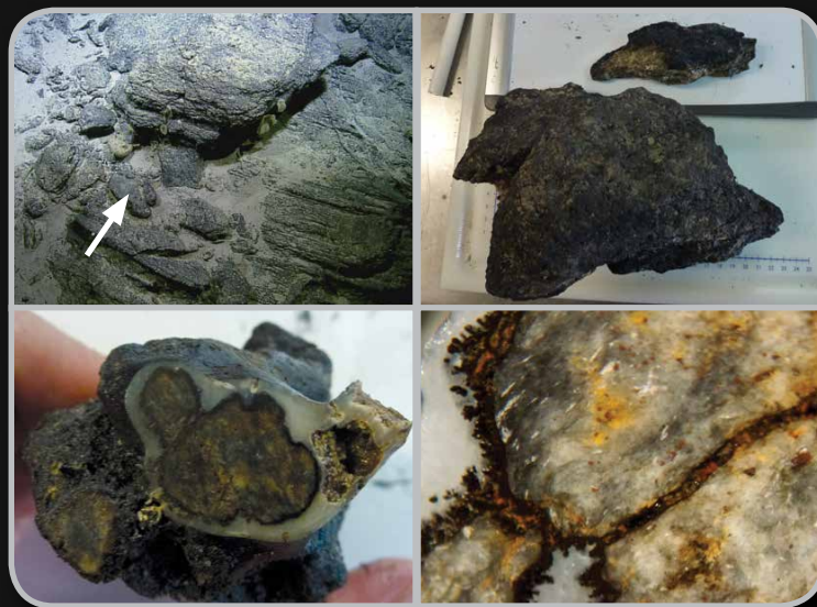
Figure 4. Several different images of the same rock sample collected by ROV Hercules (top left) to provide context. Intact in the Wet Lab (top right). Interior after cut with the rock saw (bottom left). View from a microscope to look at minerals and other features (bottom right).
