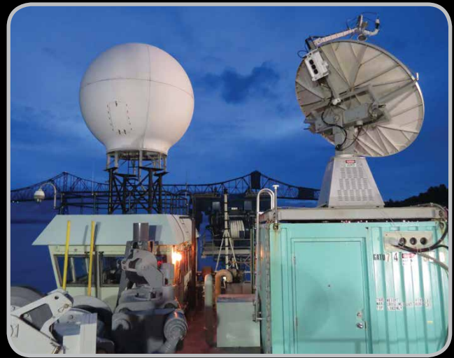
Figure 2. Final setup of the fly-away satellite tracking antenna (right), shown next to Atlantis' HiSeasNet satellite antenna system (left), during mobilization in Astoria, Oregon.
