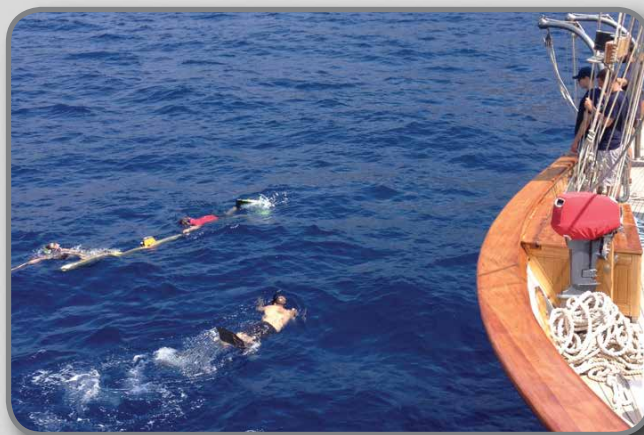
Figure 5. Launching the AUV from STS Bodrum involved lowering the vehicle from the davits on the ship's starboard side and moving it away with team members either in the water or in the Zodiac before it began its programmed mission.
