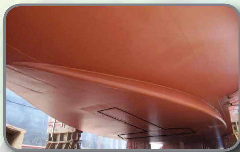
Figure 1. E/V Nautilus hull in drydock after installation of two 9 m multibeam transducers (outlined in black) that can form more than 400 beams as narrow as 1°.
