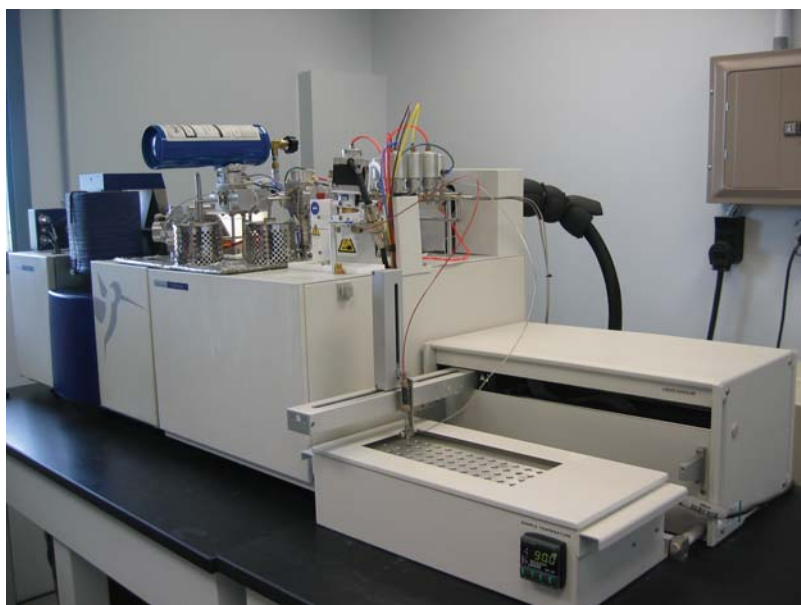
Light stable isotope ratio mass spectrometer housed at the University of Delaware, Graduate College of Marine Studies. The instrument is a GV Instruments IsoPrime mass spectrometer equipped with a dual inlet and a MultiPrep autosampler for the analysis of 60 calcium carbonate or water samples.
