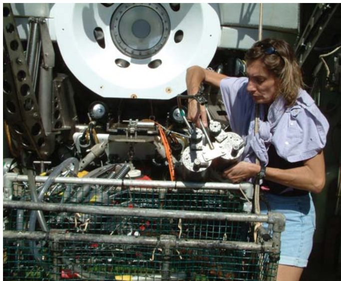
Hydrothermal vent fluids are collected in titanium bottles. After an Alvin dive, Karen removes the heavy bottles from Alvin 's basket so that shipboard chemistry can begin on them in labs aboard the R/V Atlantis .
