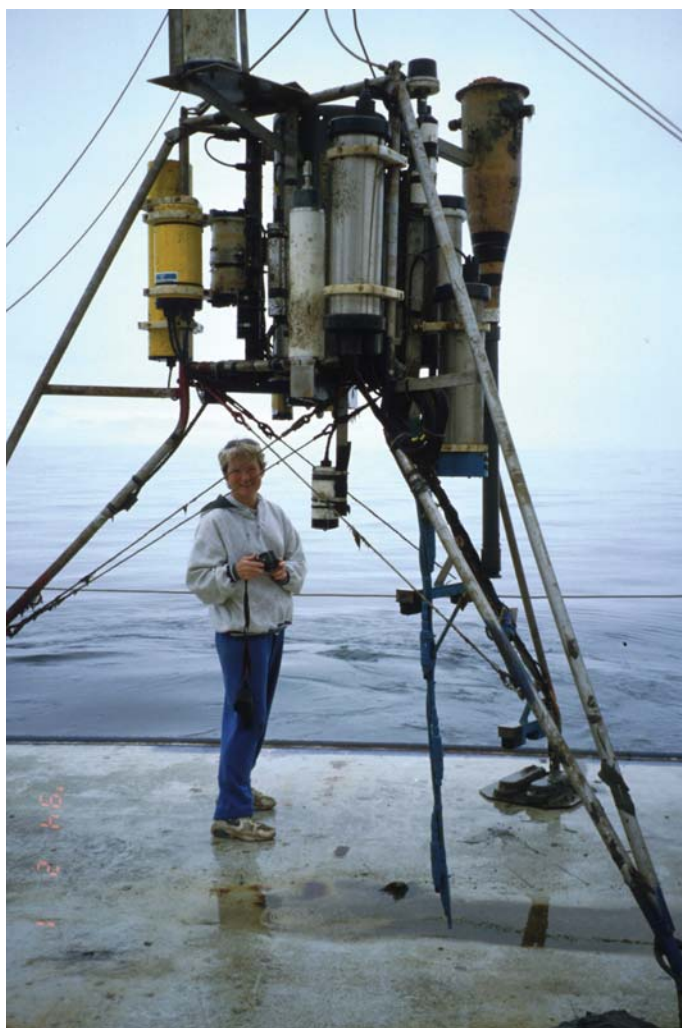
Marlene Noble next to a Geoprobe tripod designed to measure bottom suspension processes and profile currents over the entire water column. This tripod was deployed for four months in 60 m of water off Huntington Beach, CA.
