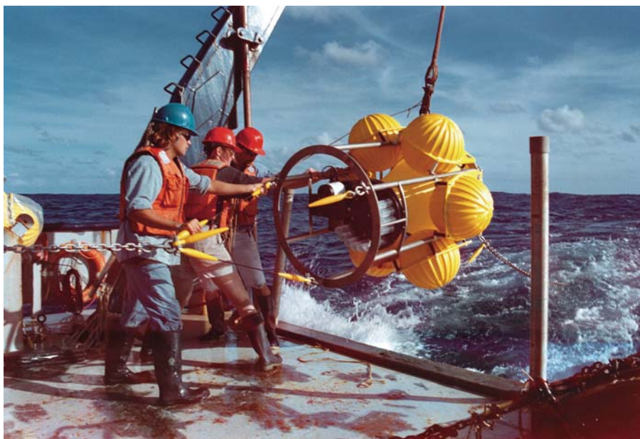
Maureen Conte (center) deploys a sediment trap at the Oceanic Flux Program time-series site off Bermuda. The OFP has produced a nearly thirty-year continuous record of sedimentation patterns in the deep ocean. Recent studies have shown the important role of transient upper ocean physical and biological forcing and of midwater biological processes on the magnitude and composition of particle fluxes.
