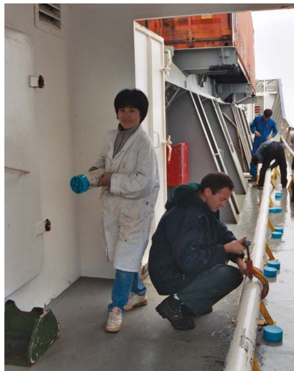
Onboard sampling during cruise P.I.C.A.S.S.O. on the research vessel Marion Dufresne . The retrieved giant piston (CALYPSO) core is cut to sections. Photo by Brooke Olson.
