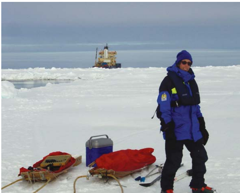
Paty sampling the microlayer of an Arctic lead at 89°N for possible atmospheric particle precursors during the Arctic Ocean Expedition-2001. The expedition was funded, in part, by the National Science Foundation. The need for clean air conditions required, at times, that the equipment be pulled with skis and sleds. The Swedish Icebreaker Oden can be seen in the background.
