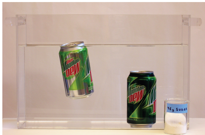
Figure 1.2. Difference in densities and, hence, sinking and floating behaviors between a can of ordinary soda (right) and a can of diet soda (left).
