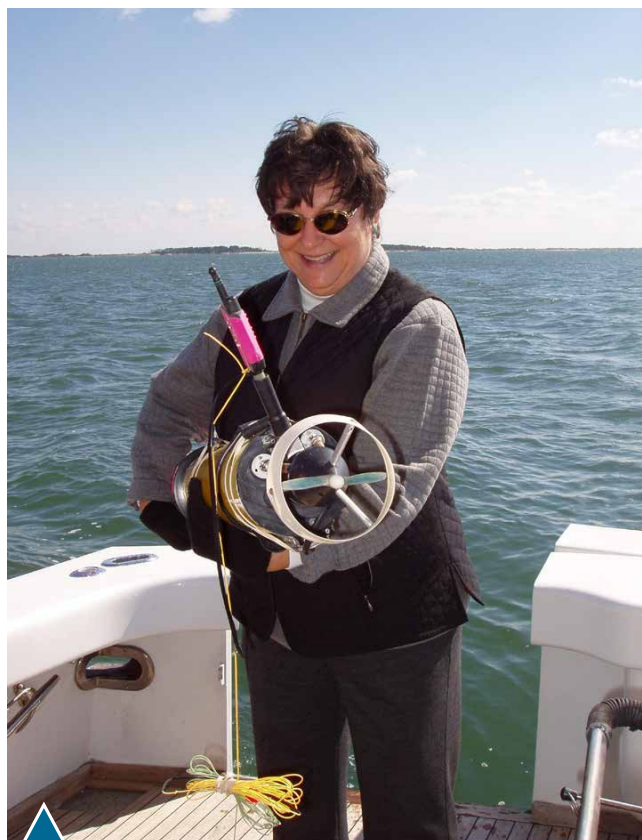
Field testing a Ranger autonomous underwater vehicle produced by Nekton Research (now iRobot) at Cape Lookout.
