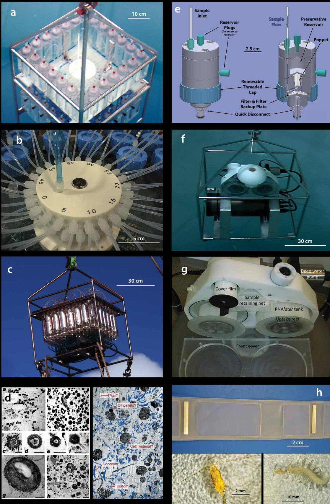
(a) A time-series Remote Access Sampler (RAS) collects phytoplankton, suspended particles, and water samples (500 ml).
